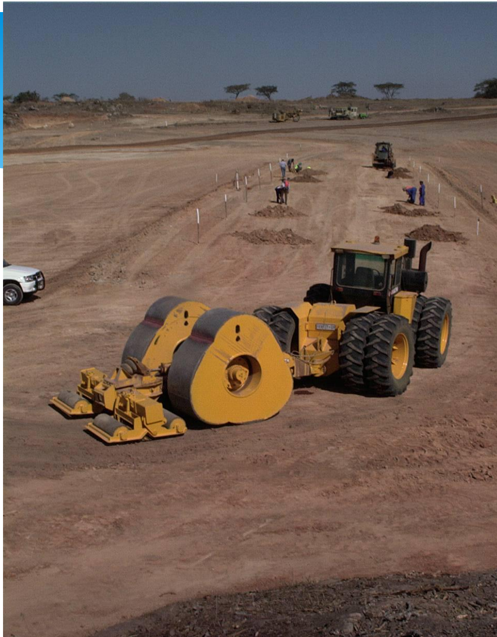
Şekil 32. 25 kJ'lük 3-yanlı darbeli silindir-Kruger Mpumalanga International Airport, Nelspruit, South Africa ( http://www.landpac.com )
